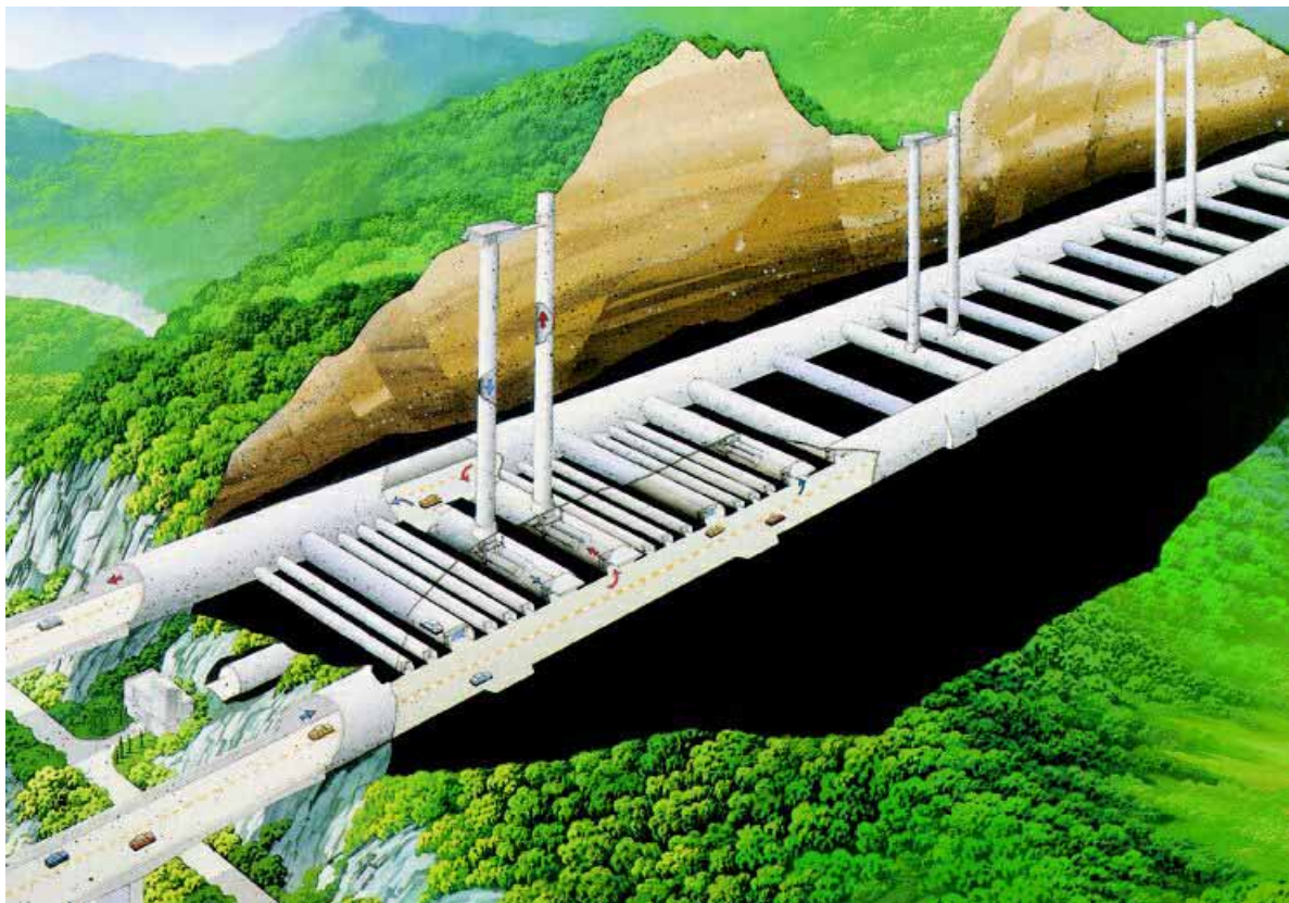
Figure 2 Ventilation System of Hsuehshan Tunnel
